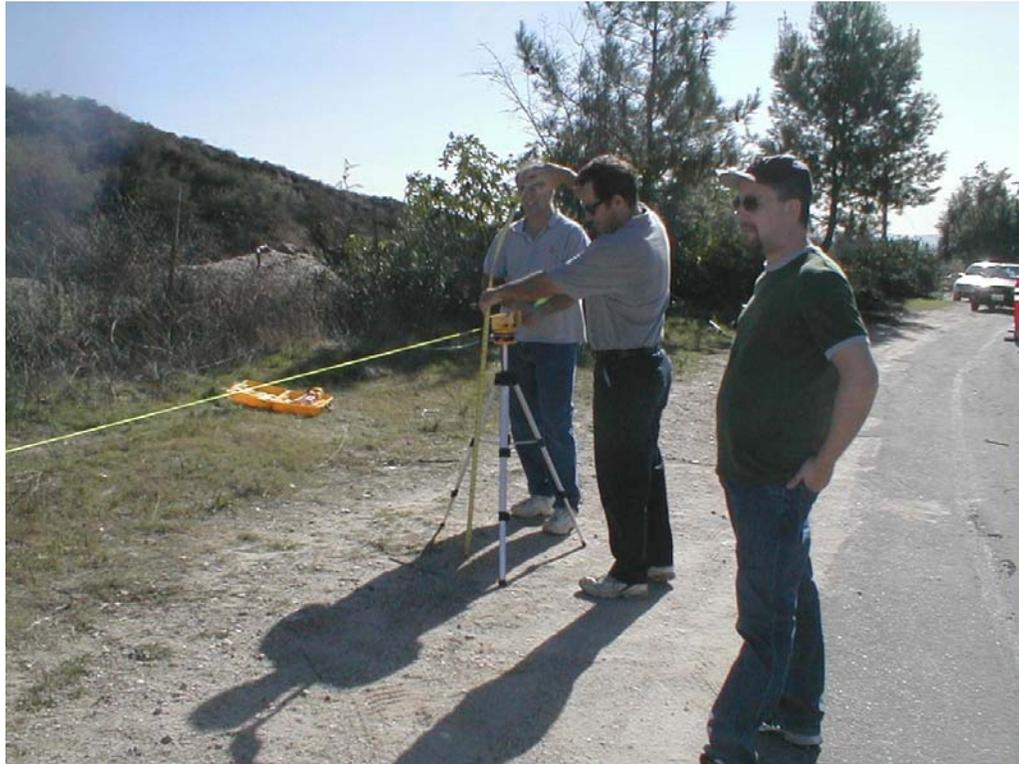
**Measuring beam height at laser**
